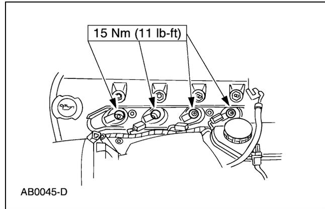
4. Inspect the spark plugs. Install new spark plugs as necessary. For additional information, refer to Section 303-00
